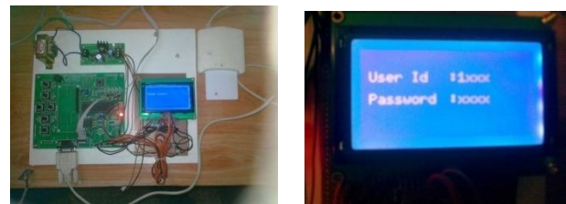
Fig.4. Input Id and password in microcontroller LCD
