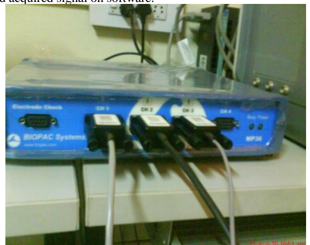
Fig. 3. Biopac MP36 biomedical data acquisition machine
