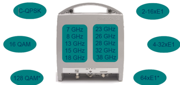
Fig.1. Radio Unit, its frequency range and modulation
