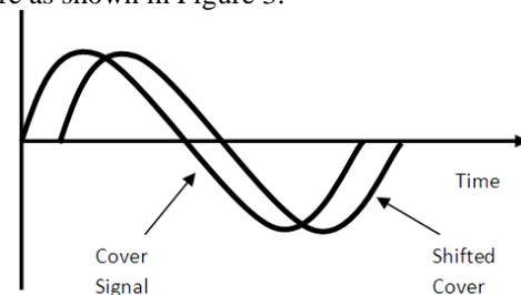
Fig.3. illustrate the original cover signal and encoded shifted signal of phase coding technique.
