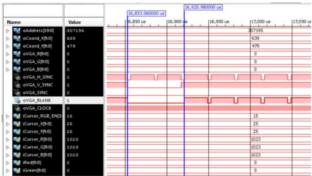
Fig. 3.7. Simulation result of VGA Controller.
