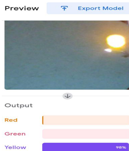
Fig. 6. Testing of the trained model using the yellow LED.
