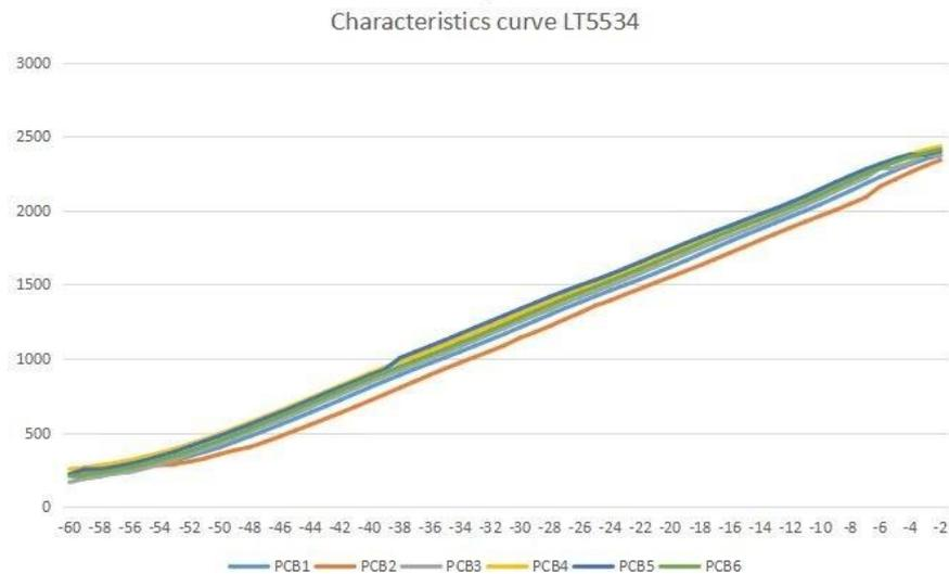
Fig. 2. Characterization curve of LT5534.
