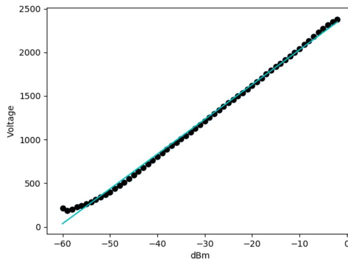
Fig. 3. Linearity from Linear regression of LT5534.
