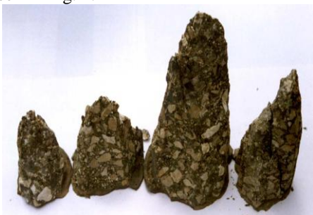
Fig.2. Specimen of High Performance Concrete after rupture
