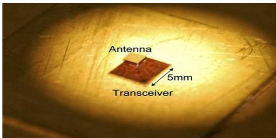
Fig. 3. Gi-Fi transceiver chip with 1mm<sup>2</sup> antenna.
