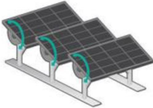
Fig. 1. Horizontal axis tracker [9]
