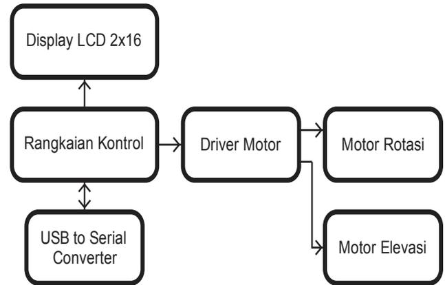
Fig. 4. Block diagram of solar tracker
