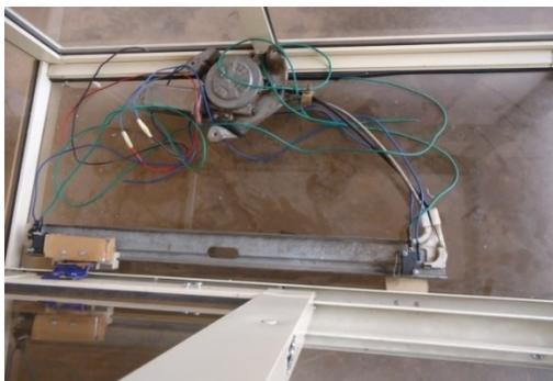
Fig. 6. Sliding mechanism for the door
