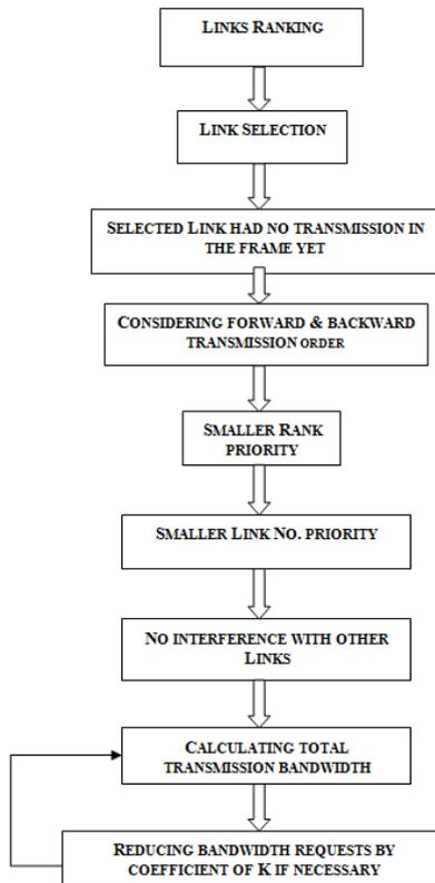
Fig. 2. Stepwise diagram of proposed algorithm
