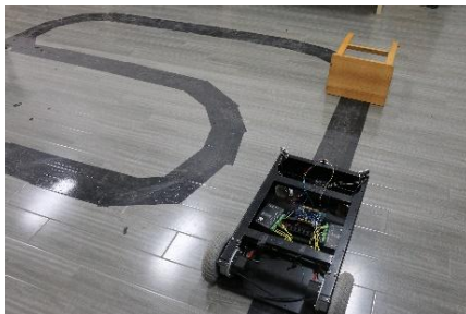
Fig.8. Mobile platform tracking test
