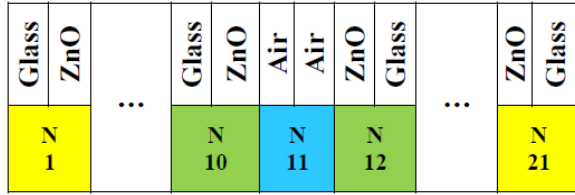
Fig.7. 21-layer periodic structure with defect
