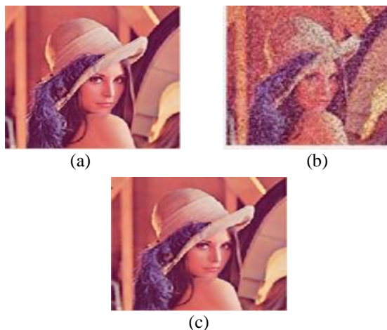
Fig.8. Execution of WSM filter - Removal of impulse noise from Lena colour 8(a) Original image 8(b) noisy image 8(c) Denoised image
