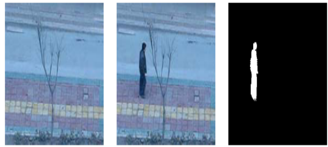
(a) Background (b) Motion Object (c) Difference Image Fig.3. Screenshot and Difference Image
