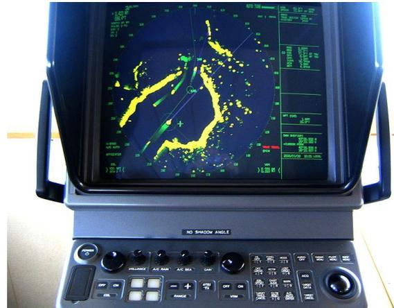
Fig.1. Electronic navigation display
