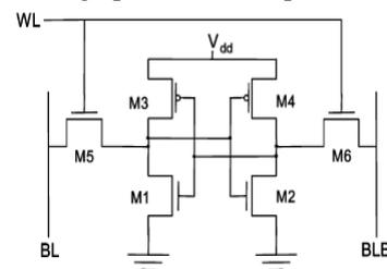
Fig.1. Conventional 6T SRAM
