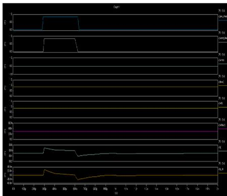
Fig.6.5: 10T SRAM Write operation
