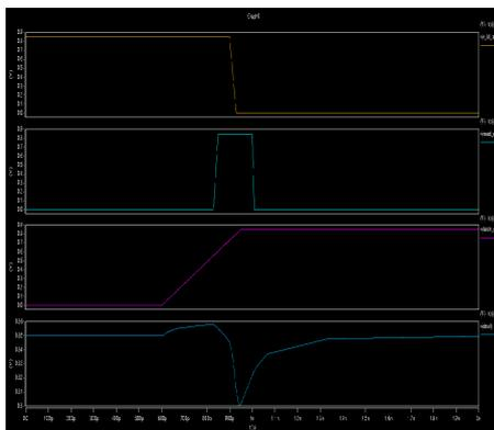
Fig.6.6: 10T SRAM Read operation
