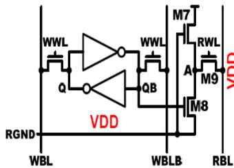
Fig.3. 9T SRAM Cell
