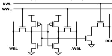
Fig.2. 8T SRAM Cell
