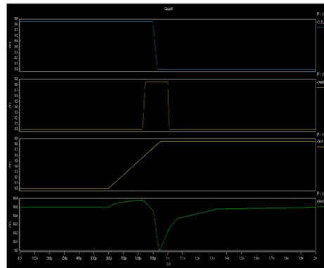
Fig.6. 8T SRAM Read operation
