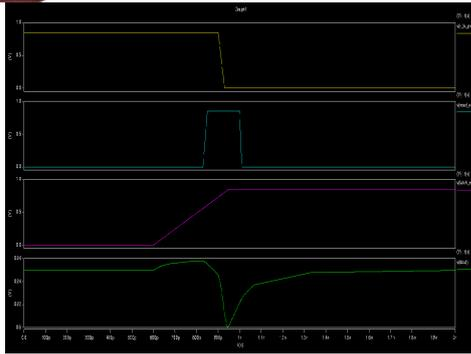
Fig.8 9T SRAM Read operation
