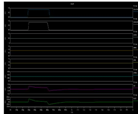
Fig.5. 8T SRAM Write operation
