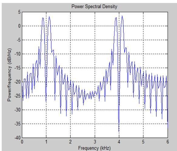
Now we're adding another User, the system will search the first available gap in the spectrum and automatically assign it to the new user. As the first available gap was after User 1 as User 2 was not sending any data so the band reserved for User 2 at start is now assigned to this new User.
