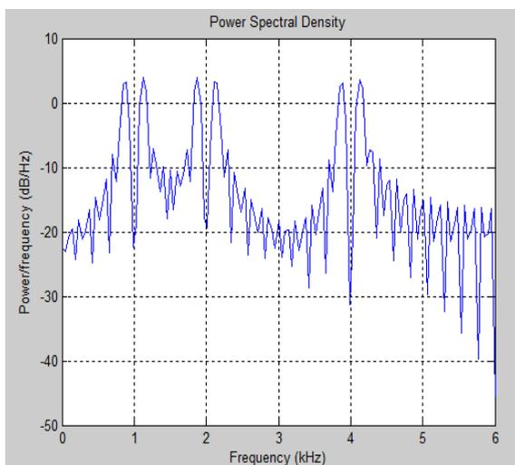
Here we can see that the first spectral gap has been filled by assigning it the new incoming User's data. The first spectral gap belonged was that of User 2.
