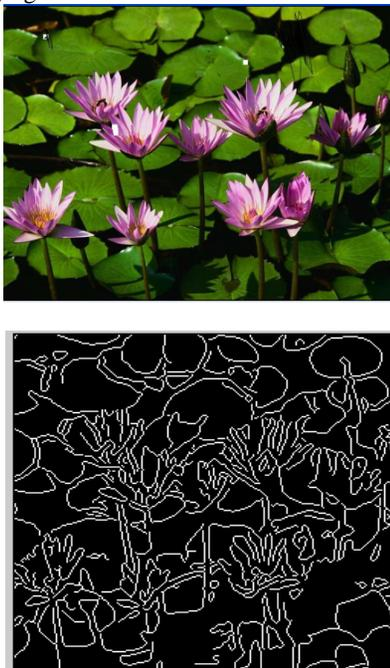
Fig.3. Example of the image transformed into edges by Canny operator
