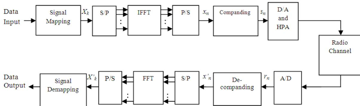
Fig.1.OFDM system using companding techniques.
