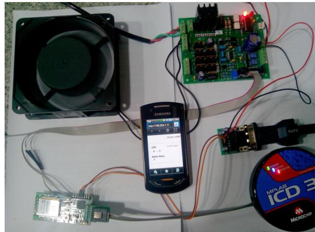
Fig.9. Monitoring & controlling the device through mobile using Wi-Fi network
