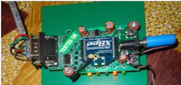
Fig.5. Zigbee Module
