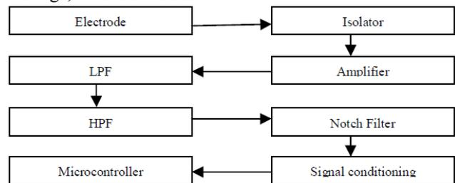
Fig.4. Block diagram of ECG system
