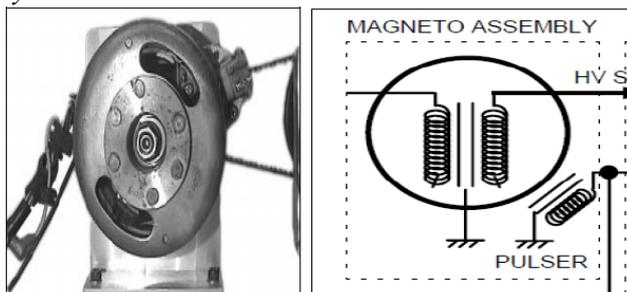
Fig.4. Magneto assembly and its coils.
