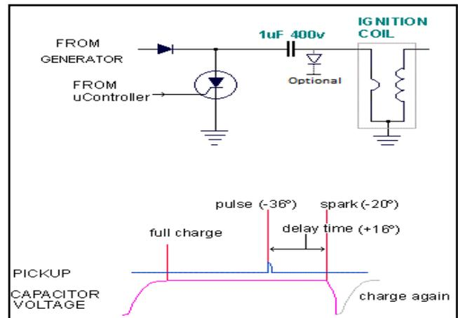
Fig.5 Element of AC CDI which shows SCR is controlled by microcontroller.
