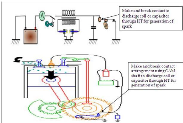
Fig.2. Electromechanical Ignition System
