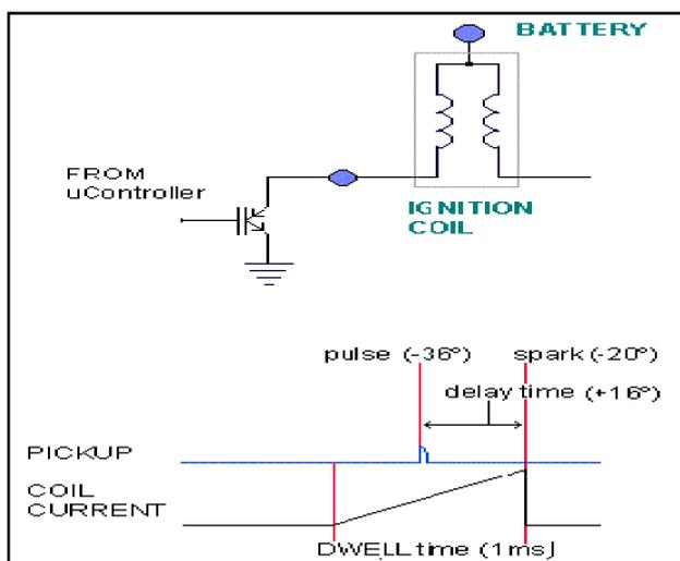
Fig.7. TCI (Transistor Control Ignition)
