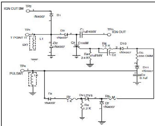
Fig.3 Electronic Ignition System with Solid-State Device (SCR- C106M)
