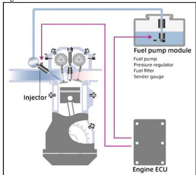
Fig.8 Fuel Injection System
