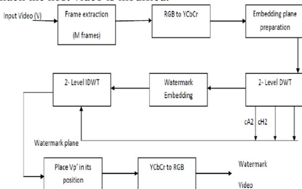
Fig.1. Watermark Embedding Algorithm
