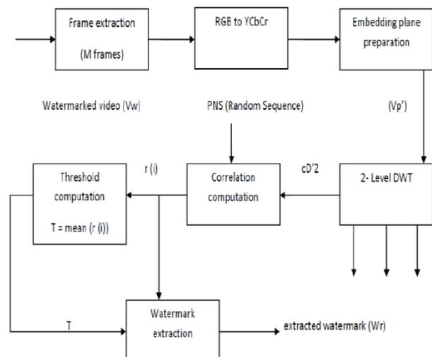
Fig.2. Watermark Extraction Algorithm
