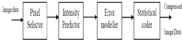
Fig 1: Block Diagram of data flow
