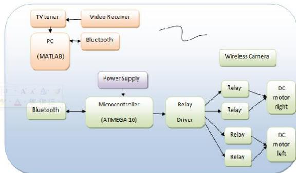
Fig.1. Hardware Block diagram
