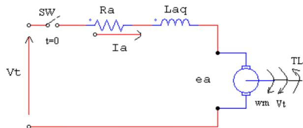
Fig.3. Schematic Diagram of DC Motor [2]
