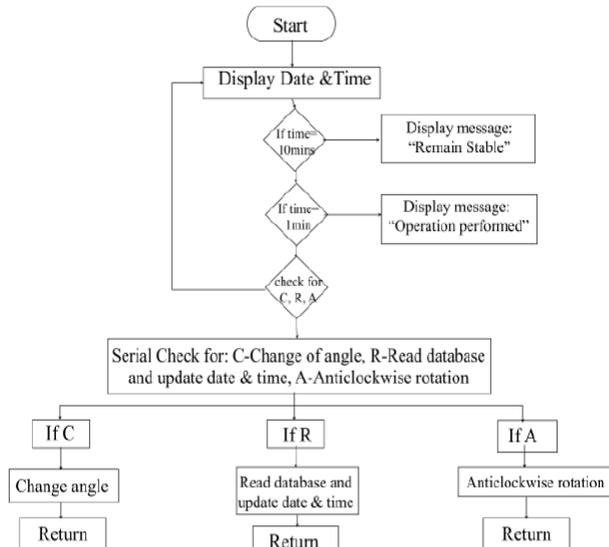
Fig.7. Flow of the hardware system
