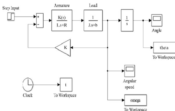
Fig.4. DC Motor Closed Loop System
