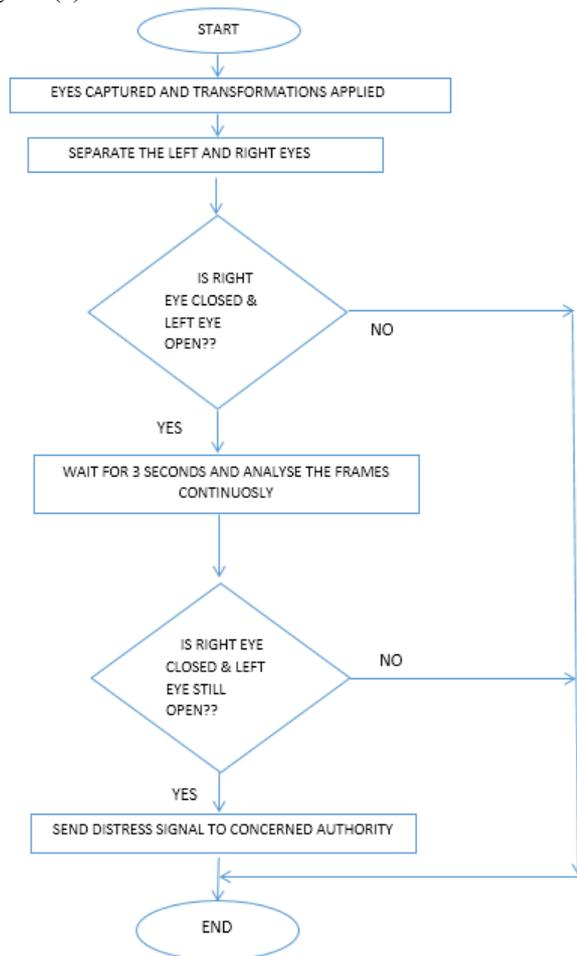
Fig.2. Identification of distress signal flow.
