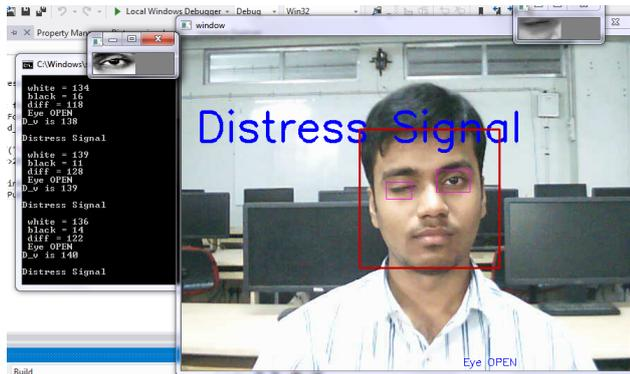
Fig.13. Results of real time distress signal detection..
