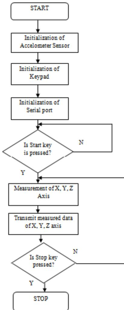
Fig.4. Flowchart of working flow of pen module
