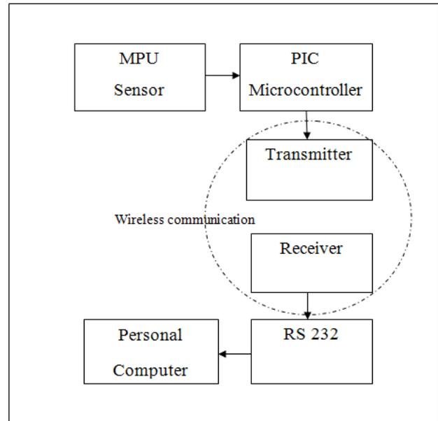
Fig.1. Block Diagram of system device
