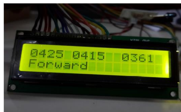
Fig.10. Co ordinate x, y, z values respectively of the accelerometer when tilted in forward direction.
