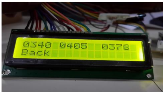
Fig.13. Co ordinate x, y, z values respectively of the accelerometer when tilted in backward direction
