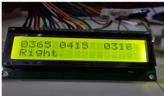
Fig.12. Co ordinate x, y, z values respectively of the accelerometer when tilted in right direction.
