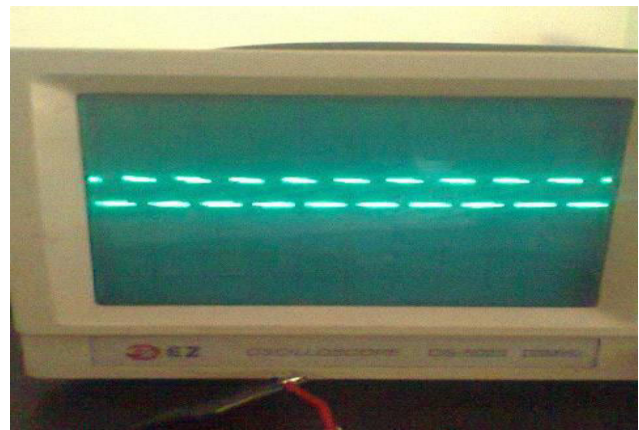
Fig.8. PWM waveform for 50% duty cycle
