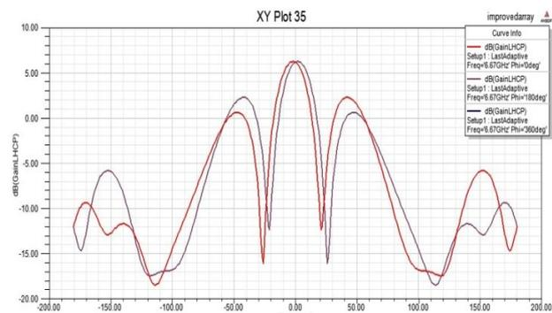
Fig. 6. Peak gain of 6.6 dB for LHCP at  $\phi = 0$
