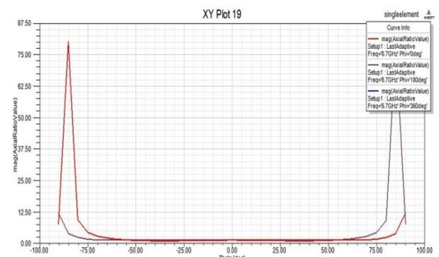
Fig. 5. Axial ratio of proposed antenna having value less than 3 dB
