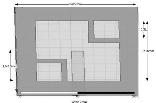
Fig. 1. Geometry of single element
