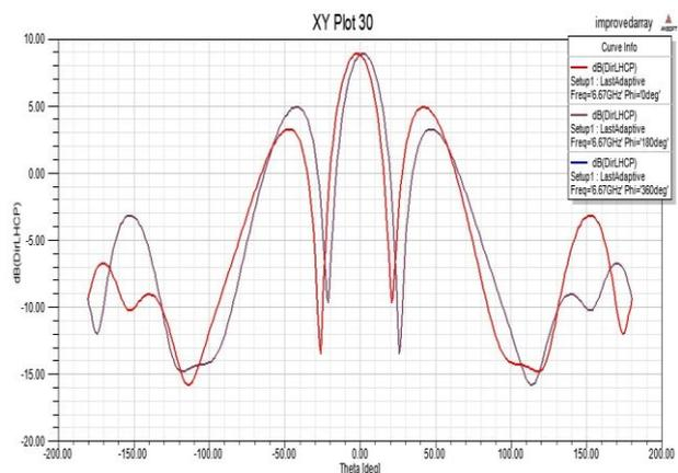
Fig. 7. Peak directivity of 9.3 dB for LHCP at  $\phi = 0$
