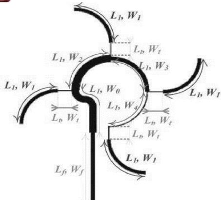
Fig. 2. Configuration of the feed network
