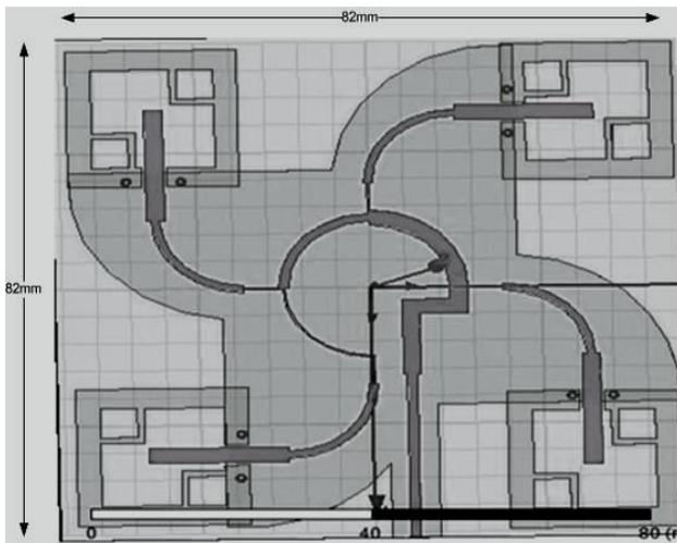
Fig. 3. 2x2 Broadband CPSSA array structure
